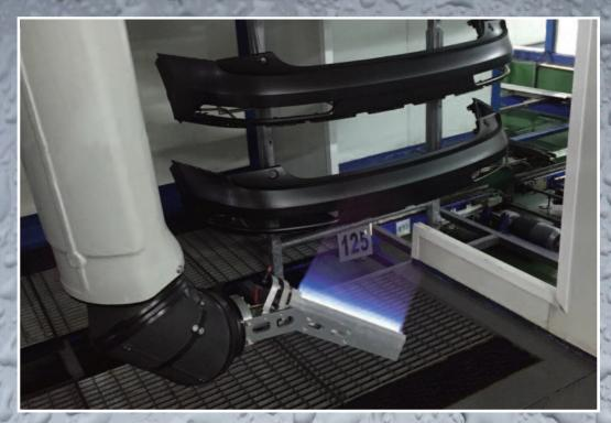
Auditable parameter, automatic air / fuel gas ratio. Equipment incorporates electronic gas flow and air flow meters and closed loop control. Parameters, alarms, interlocks and system status, shown via integrated HMI screen
